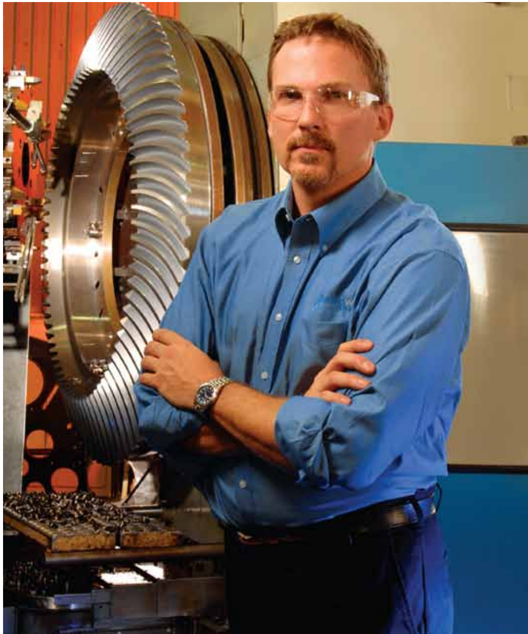
▶ The Gleason 675 bevel gear generating machine produces spiral gears up to 100" in diameter.
